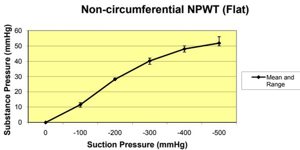
**Figure 8.** Pressure change in plasticene (mean and range when experiment repeated five times) in relation to increasing suction pressure (non-circumferential NPWT).
