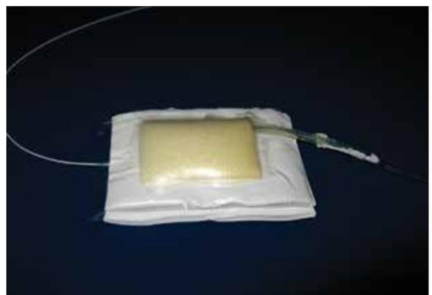
**Figure 4.** Two slabs of soft plasticene with pressure transducer in between and NPWT dressing over one slab.
