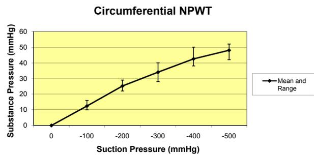
**Figure 7.** Pressure change (mean and range when experiment repeated five times) in sausage substance in relation to increasing suction pressure (circumferential NPWT).
