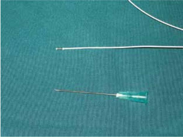
**Figure 1.** Intracranial Pressure Microsensor with standard 21-gauge needle for size comparison.
