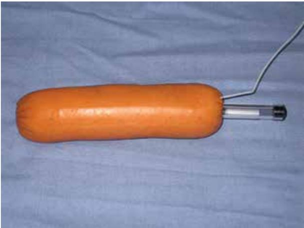
**Figure 2.** Sausage skewered onto disposable pen to represent limb/finger with underlying bone. Pressure transducer inserted to a depth of about five centimetres into substance of sausage.
