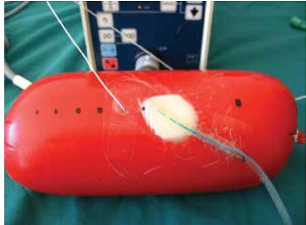
**Figure 6.** Markings at one-centimetre intervals away from cavity, at which point three pressure transducers are to be placed at a depth of one centimetre.
